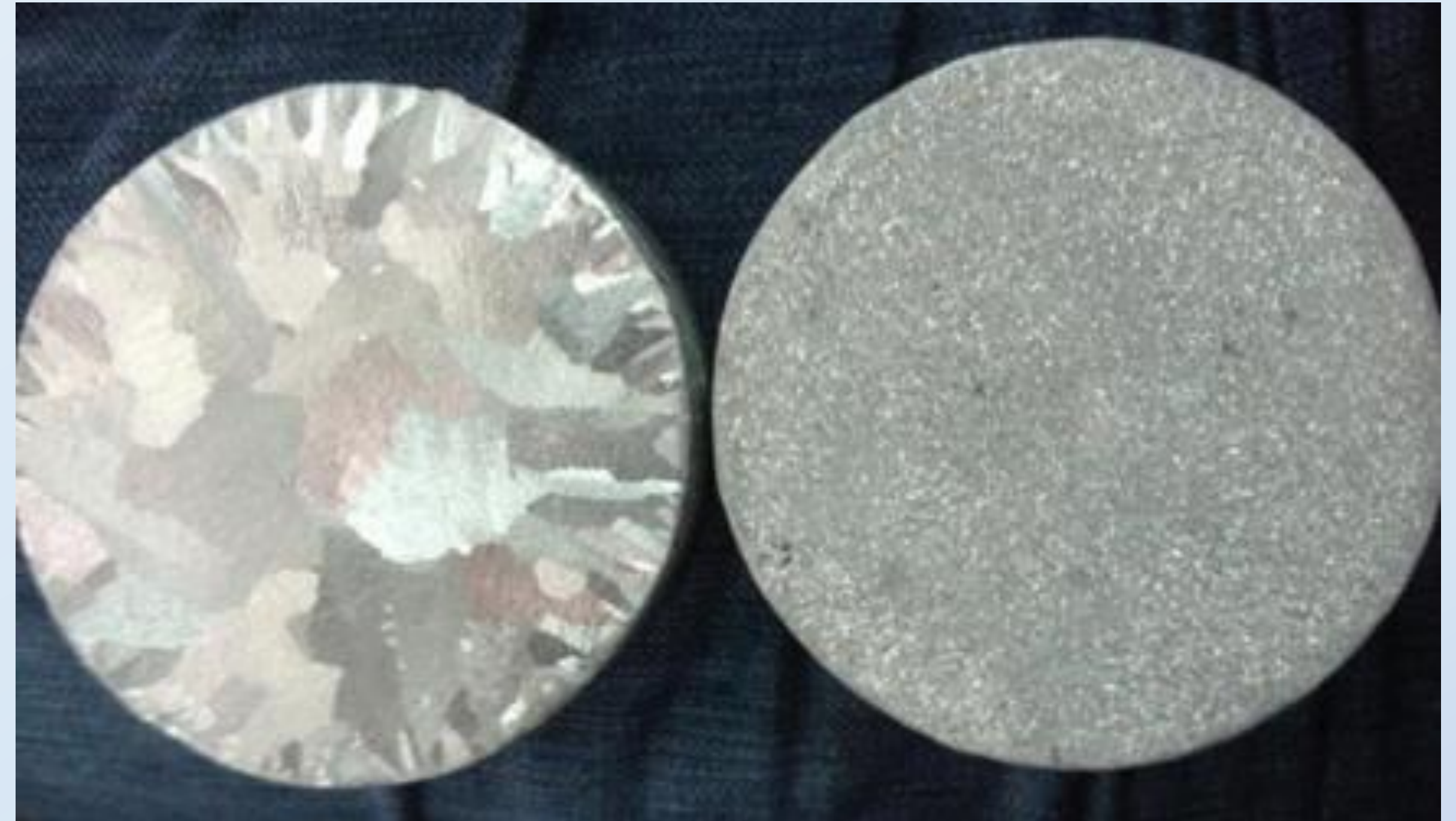
Superior Grain Refinement: Aluminum Alloy without scandium (left) and Al-Sc (right) 1
